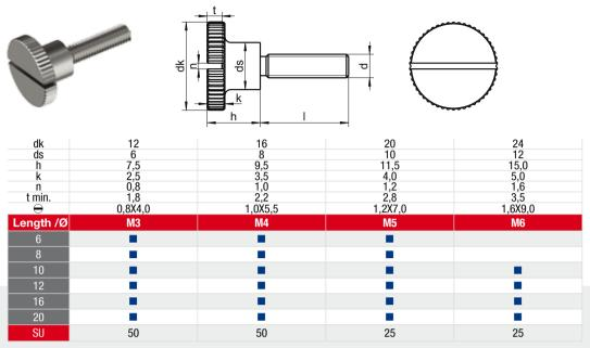
■ A1 / ▲ A2 / ● A4 | SU: Sales unit | All measurements in mm | Other dimensions on request. Example item no. 465-2-6X20 DIN 465 - A2 - M6 - I = 20mm
